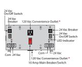
Move internal jumper to "HOT" position if you wish outlets to always be hot otherwise outlets will be switched by main breaker.\*
